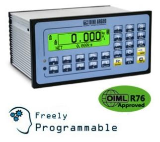
Multifunctional microcontroller/ weight indicator for use in industrial systems. 16 outputs and 8 digital inputs, 3 RS232/RS485 serial outputs, 16 bit analogue output, Sysway transmission protocols and RTU Modbus are some of the features of this indicator, which, added to the range of available application software programs, allow the use in dosage and weight verification applications, with direct management of the automation. CE-M approvable (OIML R-76 / EN 45501).
