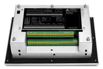
Up to 16 digital outputs and 8 digital inputs (with IOEXPB option).
