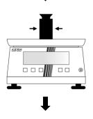
⇒ Place the calibration weight in the centre of the weighing plate
