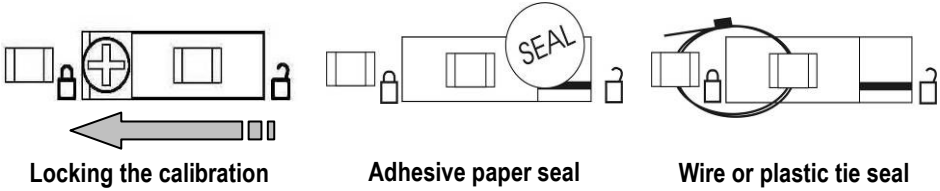
Figure 4-1. Locking and Sealing the Calibration Lock Switch.
