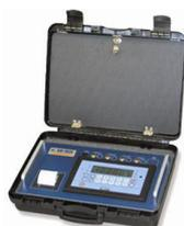
DFKWR indicator Rack version including 4 connectors for link with the platforms, built-in rechargeable battery, case and battery charger.
