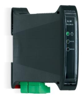
Thanks to the Hub function, PROFINET <u>interface</u> allows to convert to PROFINET protocol up to 16 independent transmitters, simplifying the installation and reducing the costs.
