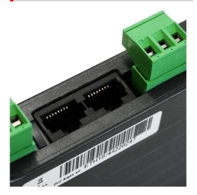
Thanks to the quick connect system, the connection between DGT1S weight trasmitter and the interface is rapid and simple.
