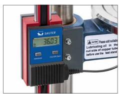
Distance measurement directly in machines or sites with RS-232 interface
