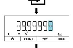
⇒ Enter the value for the specific density of the auxiliary medium (unit g / cm³; for numerical input, see Chap. 3.2.2)
