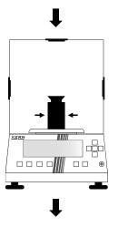
⇒ Place the calibration weight in the centre of the weighing plate
