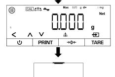
⇒ Weight value is saved (the number at the bottom left shows the number of weighings)
