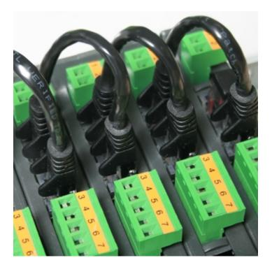
The Quick Connect System simplify and speed up the connection between DGT1S weight transmitter and this interface.
