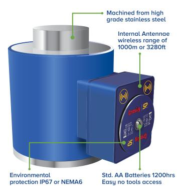
The Straightpoint LoadSafe Compression Loadcell.
