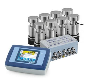
Analogue weighbridges kit made up of 3590ET touch screen weight indicator with AF03 software for weighbridges, 8 stainless steel IP68 "RCPT" analogue load cells, complete with galvanized steel oscillating resting joints and equalisation box with surge arresters.
