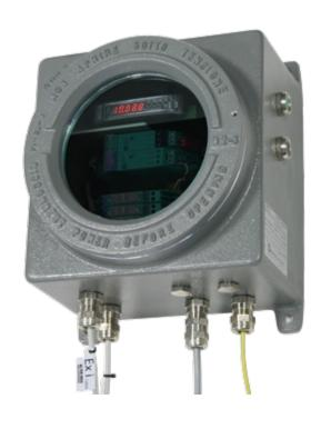
Box with Exd protection completed with weight indicator/transmitter, Zener barriers and intrinsically safe 4-20mA analog output. Fitted with 2 buttons for the main weighing operations with configurable functions, and two programmable electronic outputs for setpoints and levels management. Complete protection:
