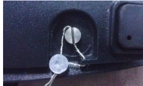
Locked with Wire Seal
