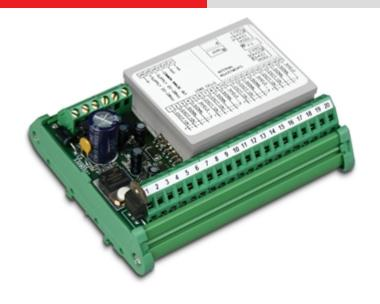
Weight transmitter with 0-20mA, 4-20mA, 0-10Vdc or +/- 5Vdc analogue output at choice. Suitable for assembling on the panel rear or in tin box on omega bar. Normally used with 12-bit analogue / digital cards installed on PLC
