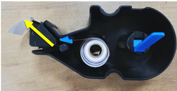
⑤ Load new receipt roll, then insert Receipt paper under the slot of winding Bobbin
