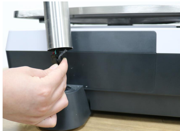
④ Insert pole with cable to the holder
