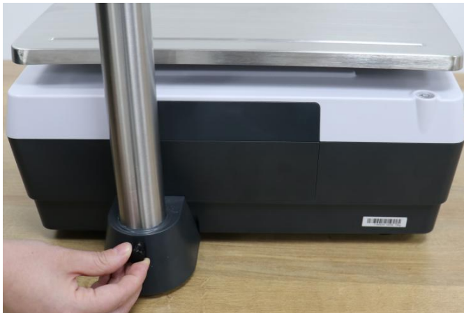
③ Take the cable connectors into the pole
