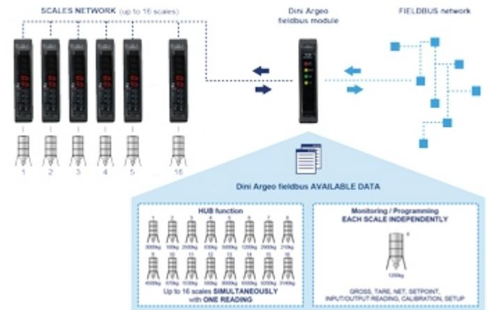
PROFINET FOR DIGITAL WEIGHING SCALES: CONFIGURATIONS
