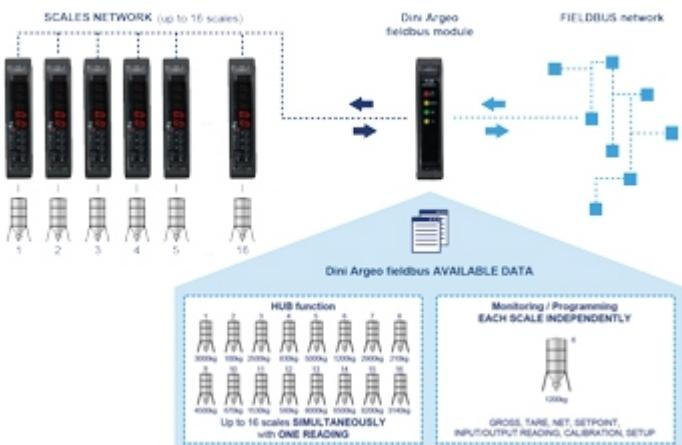
ETHERCAT FOR DIGITAL WEIGHING SCALES: CONFIGURATIONS
