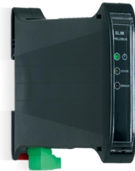
The ETHERCAT interface allows the communication among 16 different digital weighing scales at the same time, reducing the costs and the complexity of the weighing system.
