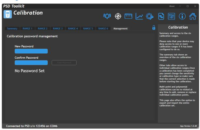
Allows setting a new password or removing an existing password to protect or release the calibration settings.
