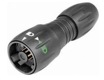
To attach this connector to the handheld, align the white arrow on the connector with the white line on the handheld socket then rotate the locking collar as indicated on the connector.
