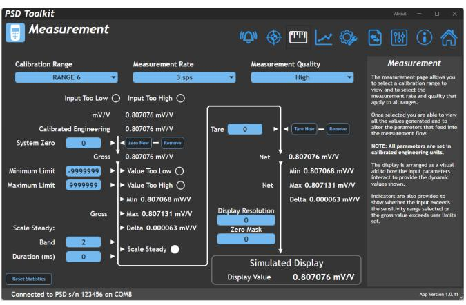
This page allows you to change the measurement settings. It is also presented in a way to visually represent how the parameters interact to generate the various dynamic result values.
