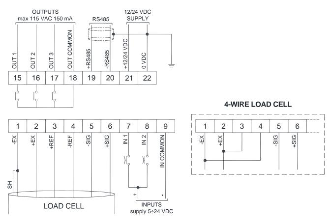
3 outputs: controlled by setpoint values or by remote device via protocol.
